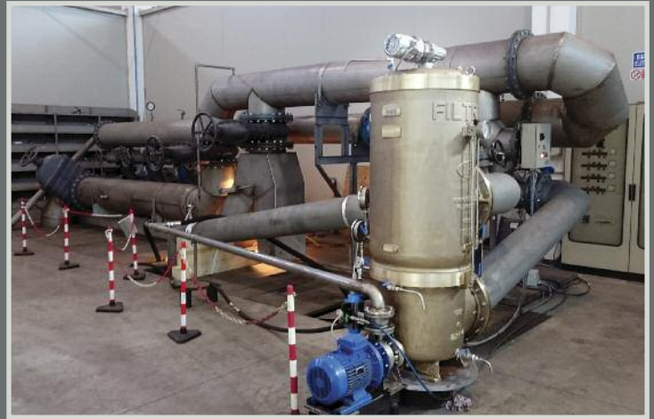
Filter ACB-9100 on test bench: Flowrates up to 4.200 m³/h
