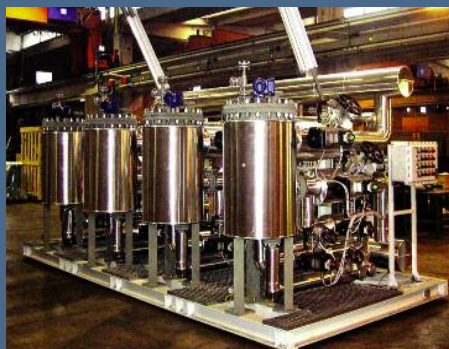
Feed Filter for DHDS Unit (Blend of VGO/LCO), Mumbai, India
