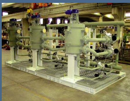
Feed Filter for Hydrocracker Unit (HCGO) - St. Charles, USA
