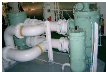
2-Stroke Diesel Marine Engine MAN B&W 6S46MC-C Ship 'SKY PRIDE' ACX-RM-SX Filter - Filtration 40 µm
