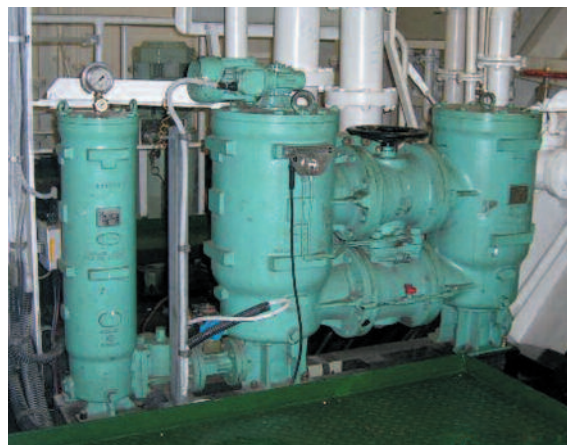
2-Stroke Diesel Marine Engine MAN B&W 6S35MC Ship "TRANS EMERALD" DACX-RM Filter Filtration 40 µm
